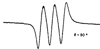
Figure 1. Derivative of the absorption ( dX^{11}/dH ) for p -fluorobenzenesulfonyl nitrene. The center of the three lines is at 8089 gauss for a microwave frequency of 9213 kMc/sec for the stated angle.
